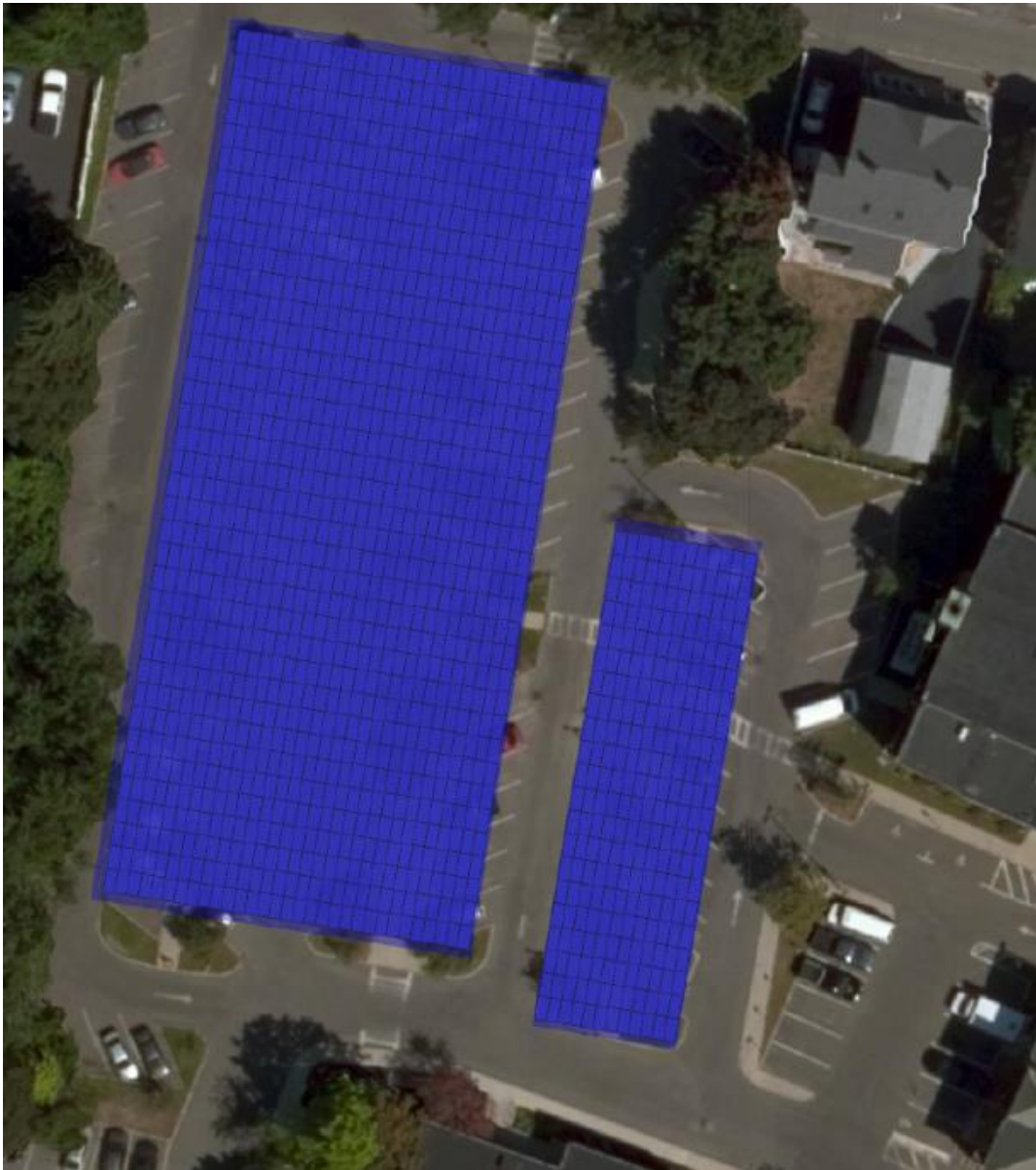
Figure 31: Proposed solar array arrangement on Plaza Parking Lot solar canopy within the Helioscope software.
